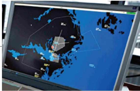
The **Saab FDP** is a safe and cost effective flight planning tool, enabling all types of flight plans to be generated, received, updated, processed and distributed in real time. Information is also communicated to external networks such as AFTN. The FDP checks the format of incoming and outgoing messages, speeding up communications and reducing the risk of human error.
