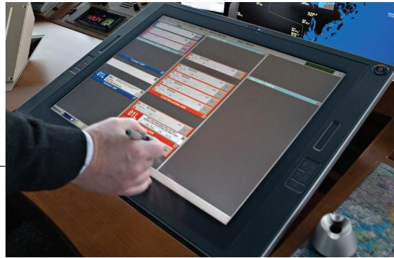
The **Saab RDP** is a reliable air situation display that can be used for providing air traffic control services for the approach and terminal volumes from the ATCT. The RDP features an intuitive and user friendly HMI that seamlessly integrates with other tower tools such as e-Strip. It supports a variety of single sensor or multi-sensor inputs and displays airborne safety nets.
